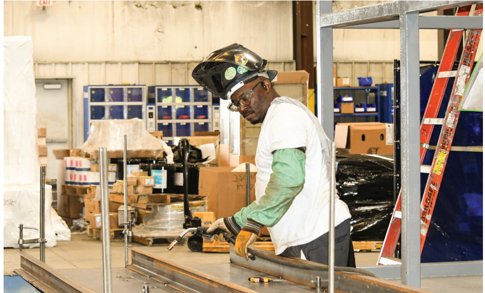
David Baker, one of Envirosep’s welders, works on a base frame.
