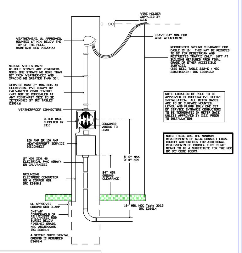
CUSTOMER POLE MUST BE 6" X 6" TREATED MIN, UTILITY TYPE POLE IS PERFERRED, SET 4" MIN. IN THE GROUND WITH A 5" MIN DIAMETER AT THE POINT OF ATTACHMENT AND ABLE TO SUPPORT A SERVICEMAN ON A LADDER. POLE HEIGHT MUST TAKE INTO CONSIDERATION THE SAG OF THE SERVICE CABLE FOR GROUND CLEARANCE, GENERALLY 1" TO 2" ADDITIONAL. MIN. POLE HEIGHT IS 12" 6" FROM FINALL GRADE
