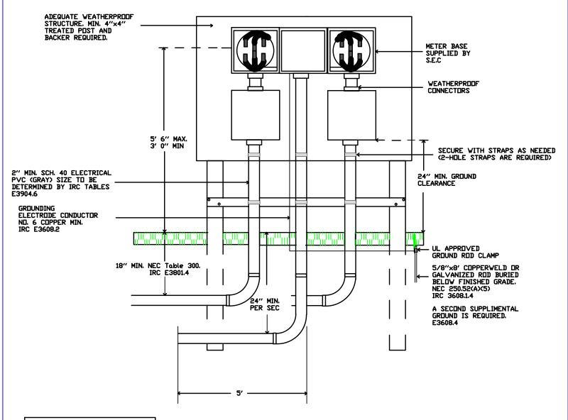
NOTE: LOCATION OF POLE TO BE APPROVED BY COOPERATIVE BEFORE INSTALLATION. ALL METER BASES ARE TO BE SURFACE MOUNTED, LEVEL AND PLUMB. ONLY ONE SET OF SERVICE ENTRANCE CONDUCTORS TO BE TERMINATED IN METER BASE UNLESS APPROVED BY S.E.C. PRIOR TO INSTALLATION.
