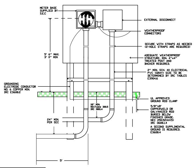
NOTE: LOCATION OF POLE TO BE APPROVED BY COOPERATIVE BEFORE INSTALLATION. ALL METER BASES ARE TO BE SURFACE MOUNTED, LEVEL AND PLUMB. ONLY ONE SET OF SERVICE ENTRANCE CONDUCTORS TO BE TERMINATED IN METER BASE UNLESS APPROVED BY S.E.C. PRIOR TO INSTALLATION.
